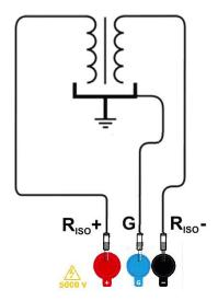
when measuring insulation resistance between one of the cable conductors and the cable jacket, the effect of surface resistances (important in difficult weather conditions) is eliminated by connecting a piece of metal foil insulating the tested conductor with G socket of the meter;
