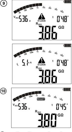
View of the screen during measurement. **DLOCK** means that the measurement was started with **ENTER** button or by pressing and holding **START** button for approx. 5 sec.
