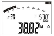
Resistance  $R_{ISO}$  value, measured in time t=5'30'. Symbol  $r \frac{11}{20}$  indicates the selected time interval, in which the resistance value was recorded.
